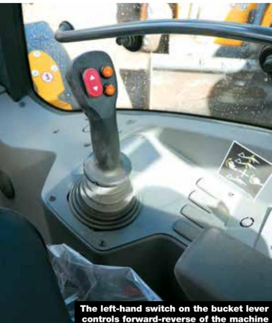
The left-hand switch on the bucket lever controls forward-reverse of the machine
