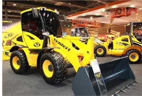
VF Venieri, which makes loaders, backhoe loaders and articulated backhoe loaders, introduced rounded bonnets in the late 1990s, says Rava, while its competitors still had square ones. Though this was partly an aesthetic decision, it also improves visibility for the driver with a better site line between the cab and ground level. Venieri’s positioning of the exhaust and the air intake close to the corners of the cab also aims to optimise the driver’s view and hence safety, say Rava.
